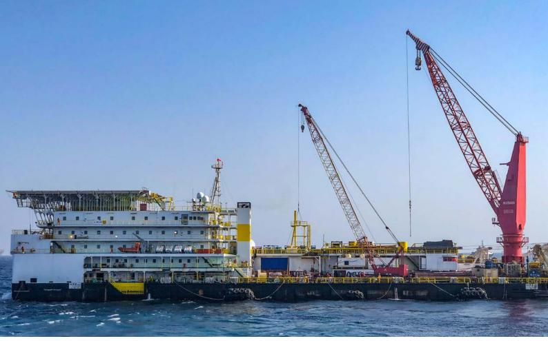
LTB 300, a pipelay-cum-work barge undertaking offshore installation
