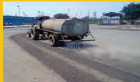
STP treated water re-used for water sprinkling in dust suppression at MFF Hazira
