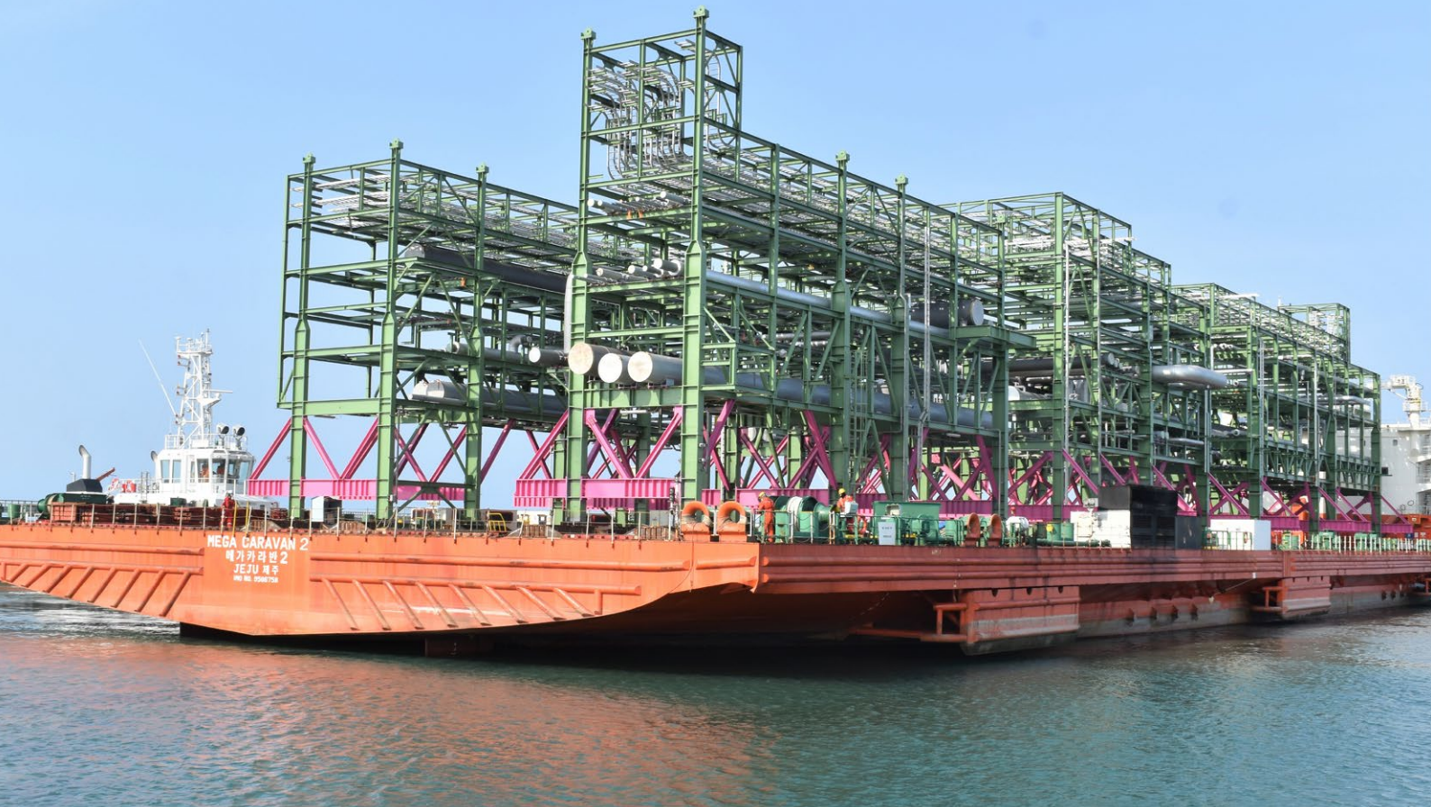
Onshore Process and Pipe Rack Modules for a leading industrial gases company.
